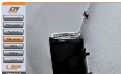
Video 1:1 tracking of the welding process and saved along with all technical parameters.
