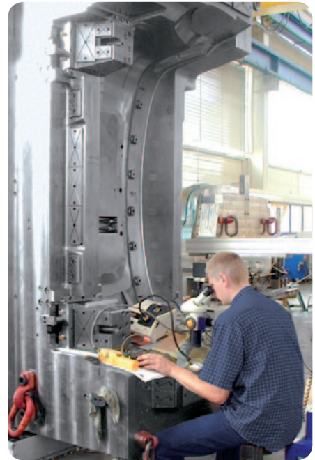
Processing of a 20 t mold for the production of automobile bumpers
